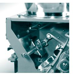
ensures optimal accessibility to the discharging element, shaft seal, and feed hopper. All steps for removal of the screw and the feed hopper can be carried out with a few grips and without the extensive disassembly of the weigh hopper.
